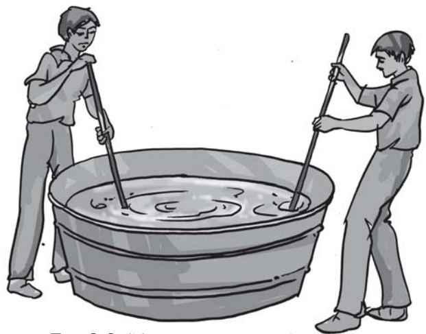
Fig. 3.8 (b) Scouring in tanks
